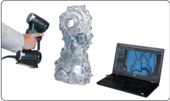
Deep hole scanning: 1 blue laser line
