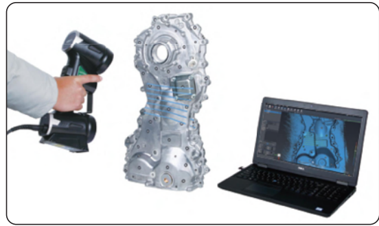
Precision scanning: 7 parallel blue laser lines
